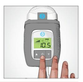
**IMPORTANT:** The "REMINDER" indicator will display on the Z1 if an air leak is detected between the Z1 outlet and the mask. This may also display at times when the mask is not being worn properly. This common condition should clear once all connections are secure, the mask is properly worn, and therapy has begun.
