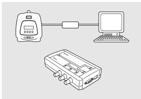
1 Connect the iSleep-iCom data cable to the iSleep 20. Make sure it is fitted correctly.
