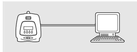
**1** Connect the data cable to the iSleep 20. Make sure it is fitted correctly.
