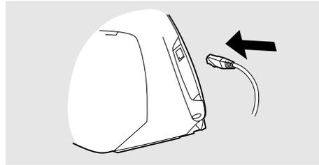
2 Connect the other end of the iSleep-iCom data cable to the iCom.
