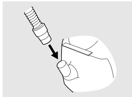
**2** Connect the other end of the patient tube to the mask and the leakage port, if applicable.
