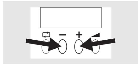
The ramp button is used to activate the ramp function during operation.
