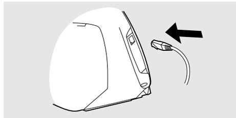
**2** Connect the other end of the data cable to the PC with the RS232 connector.
