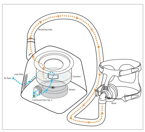
**Figure 4**Air flow from rear of device to mask.
