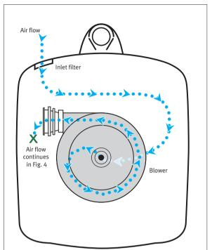
**Figure 3**Air flow from rear of device to blower.
