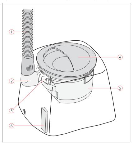
**Figure 5**Operator-detachable breathing gas pathway components.
