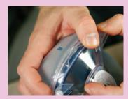
Lift up on the tabs at the bottom of the mask's integrated retaining ring.
